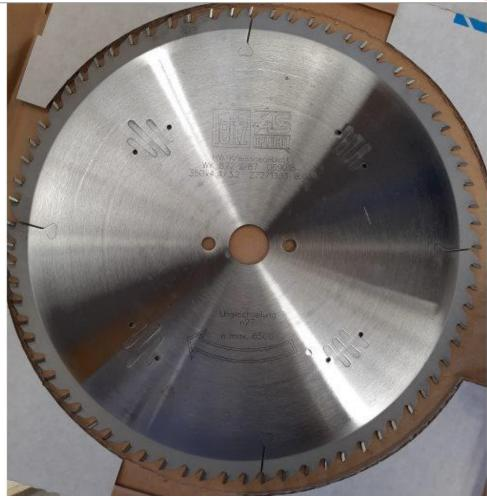
Sizing/trimming blade by Leitz. Designed for cross-cutting across grain in dry solid woods and sizing uncoated timber products and laminated woods respectively up to 90 mm cutting height. For saw benches, sizing, cut-off and multi-blade saw machines.
