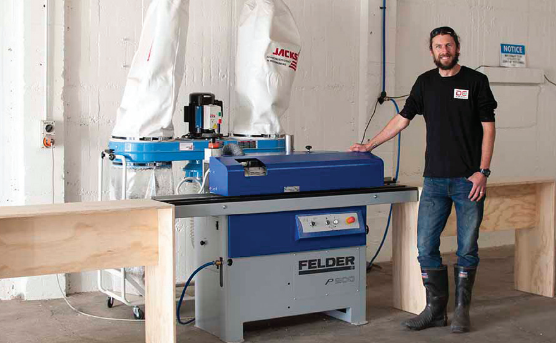
Daniel Sinclair with his Felder P200 edgebander, a compact machine for pre-glued tape and short runs.
