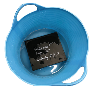
After six weeks in a bucket of water this PUR edged MDF looks as good as the day it was edged.
