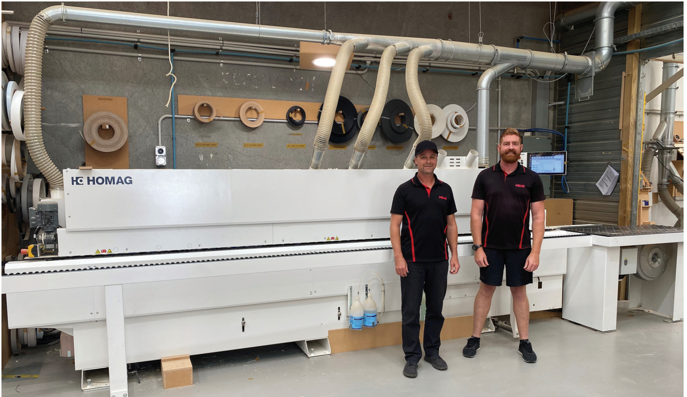
Tony Hewetson and Lance Barnes - parts now come off the edgebander with very minimal manual post-processing or cleaning required
